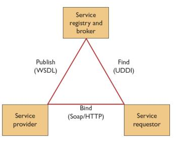
Figure 2: Basic service oriented architecture [8]
