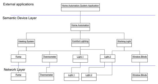
Figure 4: Semantic Devices provide a high-level programming interface.
