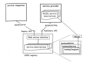
Figure 1: Basic web service architecture
